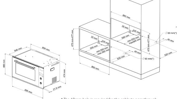
\* The 60mm hole is required for the cable to pass through
